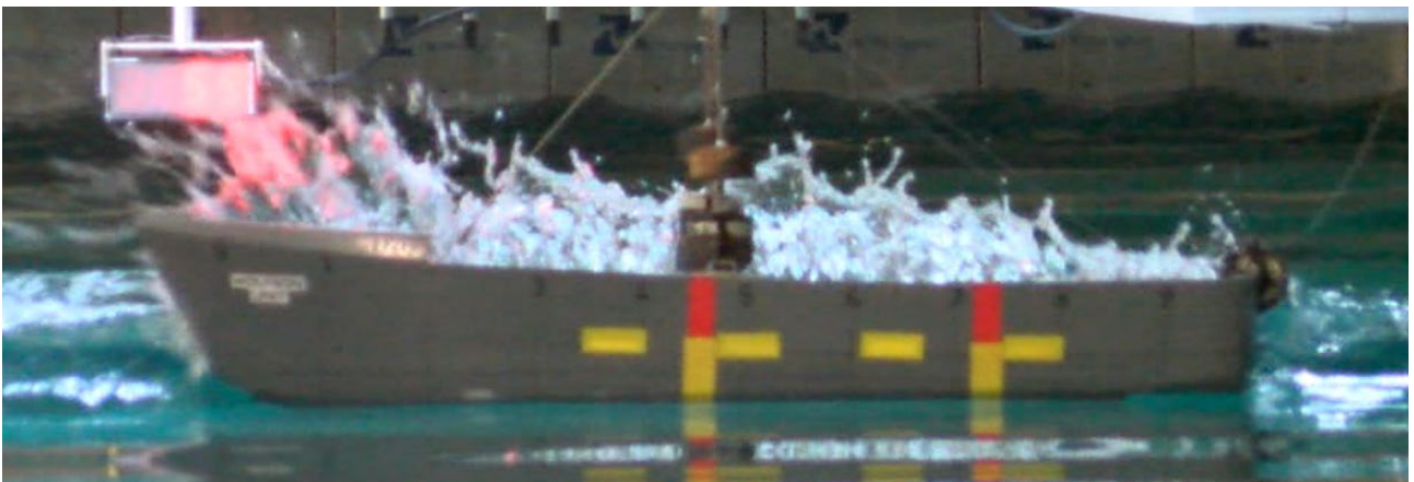
Figure 19 Open boat, loading condition 4.2, run 59: wave height 1.20 metres, wave period 2.8 seconds
